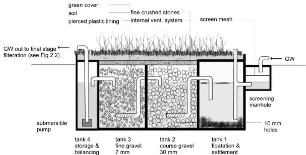
Figure 7. Physical greywater treatment system used in Qebia Village, Palestine.
