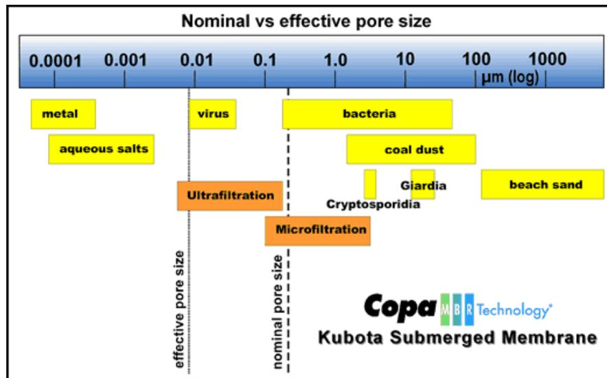
Figure 9. Membrane pore size and filtration abilities.
