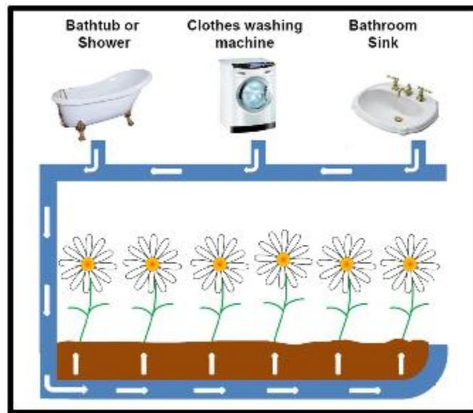
Figure 2. Schematic of typical household sources of greywater, applied to a flower garden.
