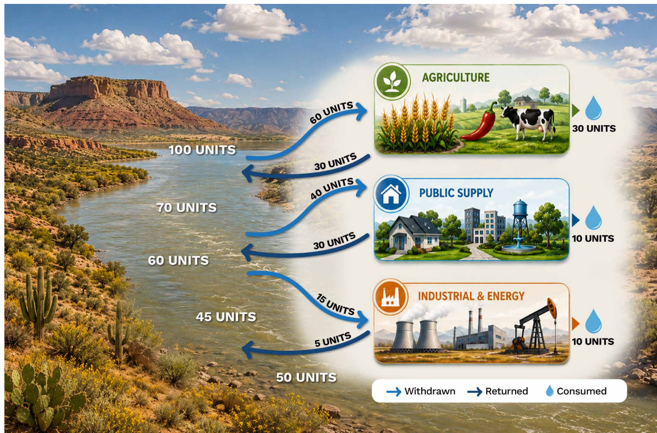
FIGURE 1: Example of water use along a river showing consumptive and non-consumptive use
