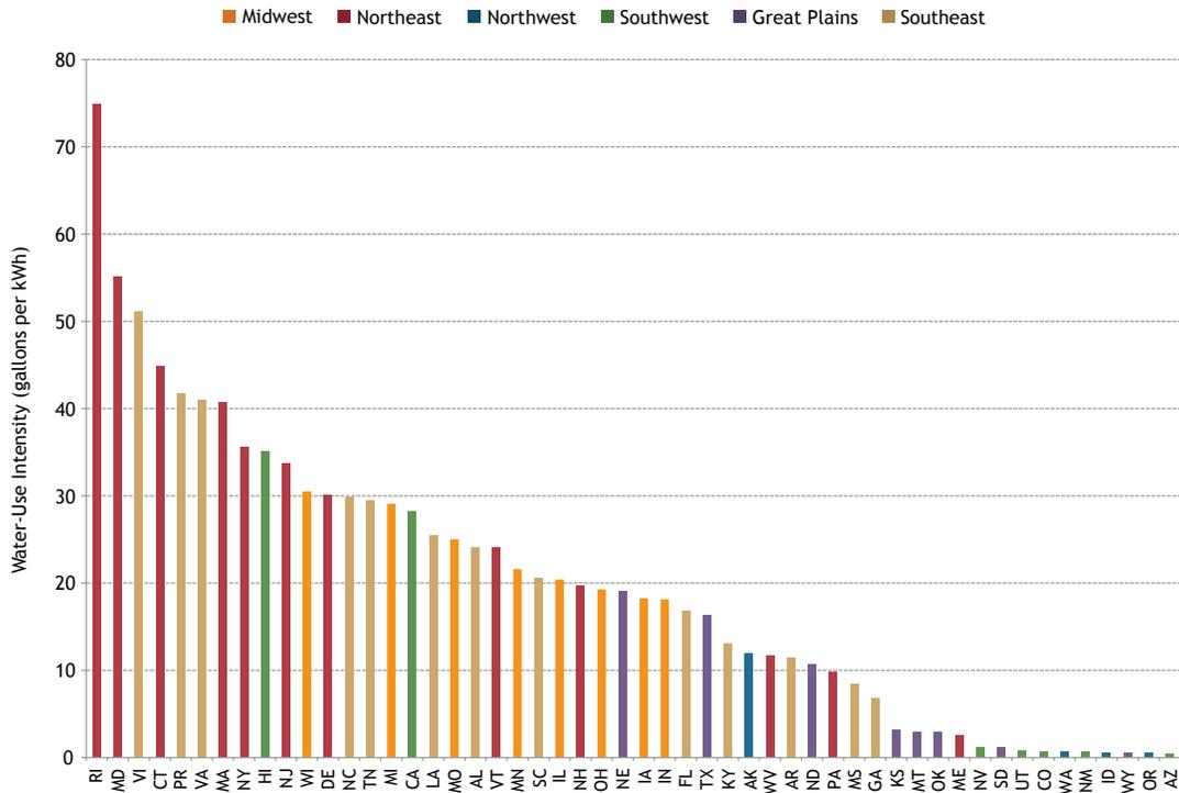
**Figure 5. Water-Use Intensity for Thermolectric Power Generation, by State (2010)**
