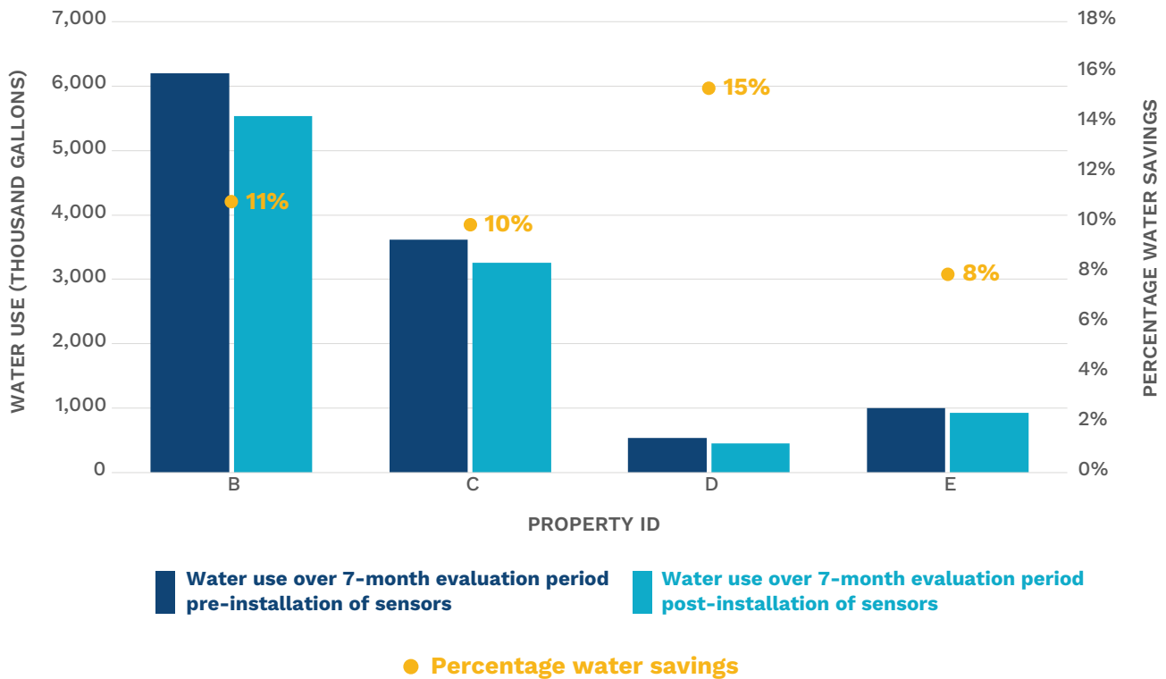
FIGURE 5. Seven-Month Water Use and Percent Savings for Four HACLA Buildings Before and After Installation of Sensor Technology
