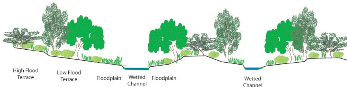
**Figure 4 Typical Cross-section with riparian plant zone.**
