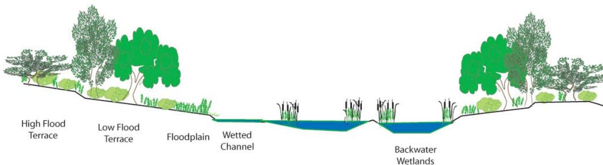
**Figure 5 Typical channel-backwater wetland cross-section**
