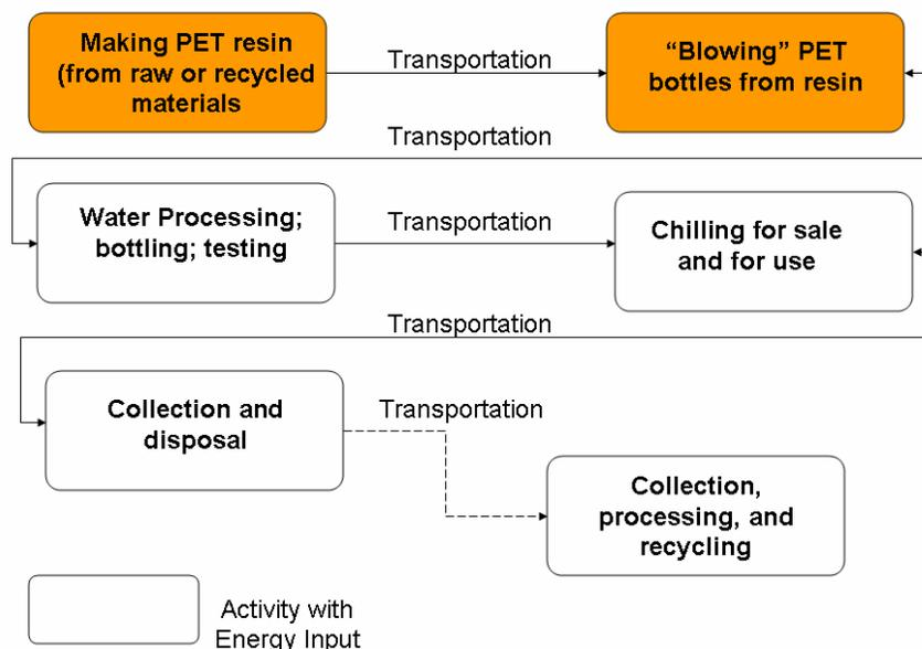
**Figure 1.** Flow diagram showing examples of where energy is required during bottled water manufacturing, use, and disposal. Energy is required at each major stage, as well as with transportation between stages. This fact sheet only analyzes the first two orange boxes, which together require the equivalent of 17 million barrels of oil.
