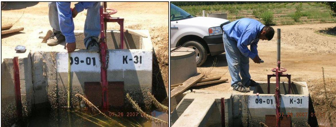
**Figure 2. District staff measuring water at a modified constant-head orifice turnout in an Alta Irrigation District canal**
