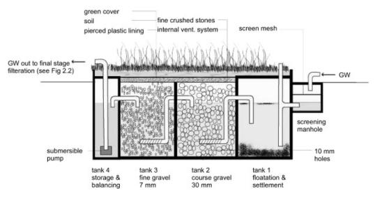
Figure 7. Physical greywater treatment system used in Qebia Village, Palestine. Source: Burnat and Eshtayah 2010
