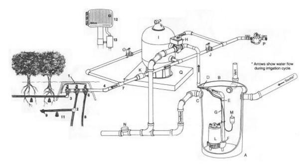
**Figure 6. ReWater's greywater treatment system for outdoor irrigation.** *Source: ReWater 2010*
