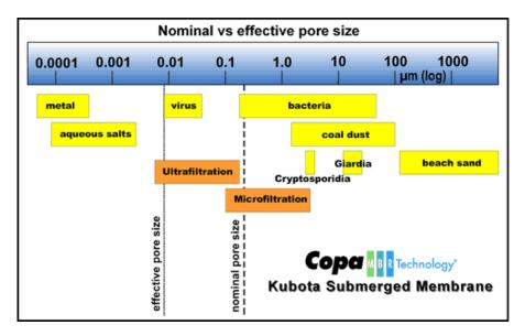
**Figure 9. Membrane pore size and filtration abilities.** Source: Ovivo 2010.
