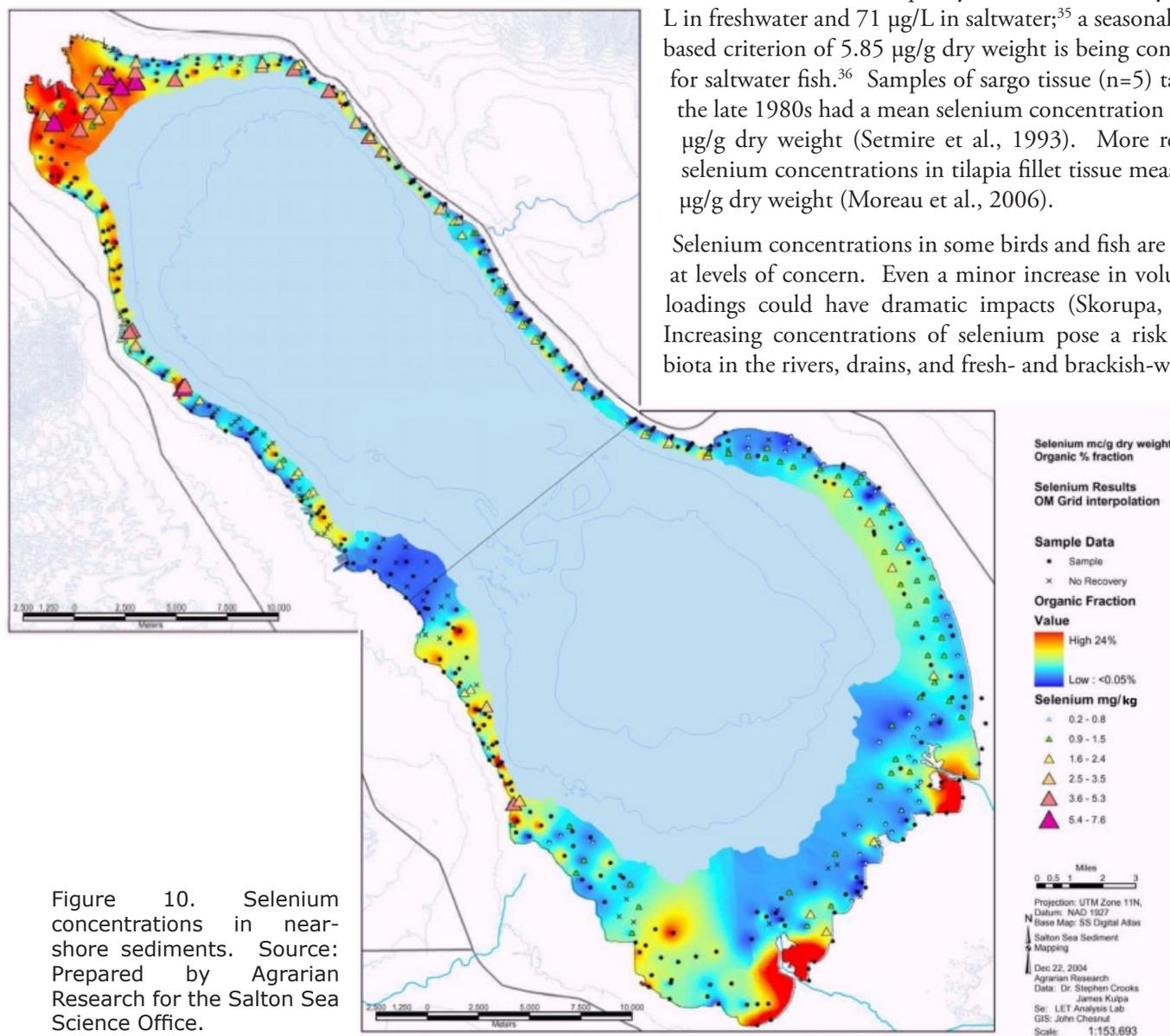
Figure 10. Selenium concentrations in near-shore sediments. Source: Prepared by Agrarian Research for the Salton Sea Science Office.
