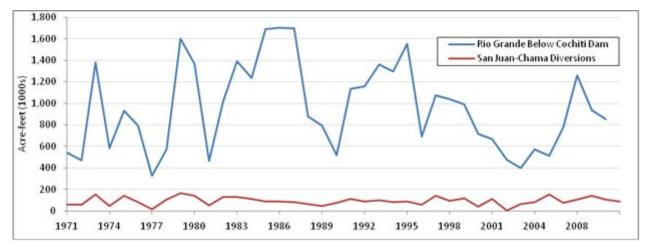
Figure 23 Annual flow of the Middle Rio Grande, including interbasin transfers from the San Juan-Chama. (Data from USGS, USBR.)
