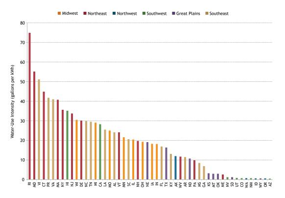
Figure 5. Water-Use Intensity for Thermoelectric Power Generation, by State (2010) Source: USGS (2014b)
