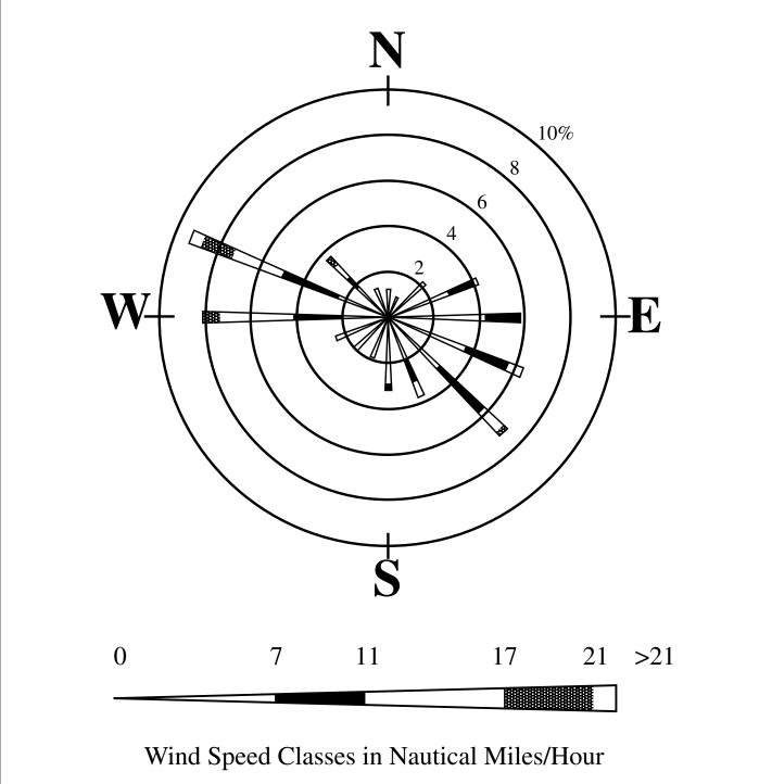
Frequency of occurrence for wind blowing from each direction. For example, wind is blowing from the west approximately 8% of the time with a wind speed between 17 and 21 knots for about 0.7% of the time.
