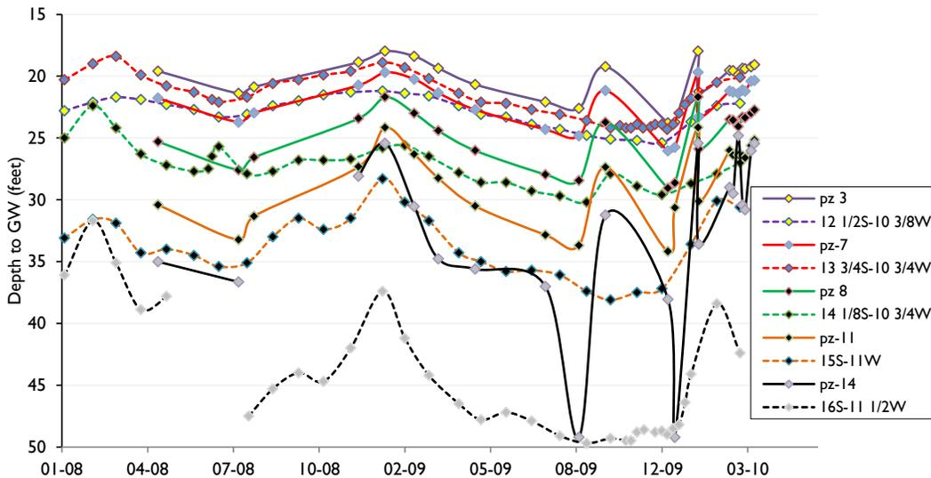
**Figure 24. Depth to Groundwater at Paired Monitoring Wells on Opposite Sides of River Channel, 2009-2010.**
