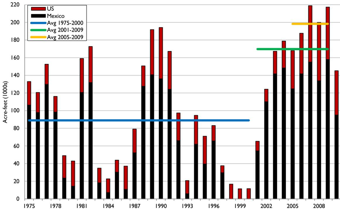
**Figure 40. Total Reported Quantity of Groundwater Pumped within Five Miles of the SIB, in Mexico and in the U.S., 1975-2010.**
