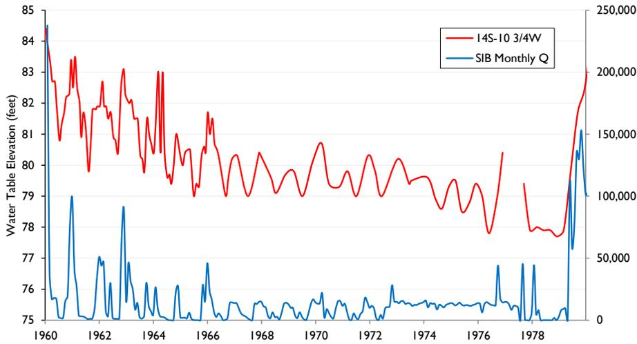
**Figure 52. Water Table Elevation near Hunter's Hole and Monthly Flows at SIB, 1960-1979.** Sources: Reclamation, IBWC.
