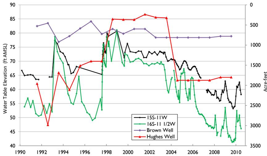
**Figure 34. Groundwater Pumping and Water Table Elevations Near the SIB, 1990-2010.** Source: Reclamation. Values on secondary y-axis in reverse order.
