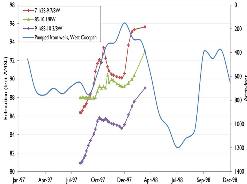
**Figure 35. Groundwater Pumping and Water Table Elevations near West Cocopah, 1997-1998.** Source: Reclamation. Values on secondary y-axis in reverse order.
