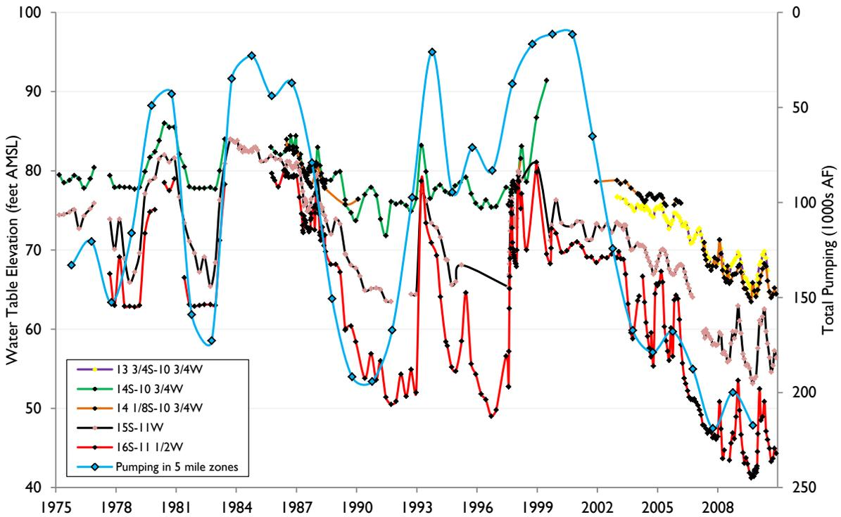
**Figure 41. Water Table Elevations and Total pumping in exclusionary zones, 1975-2010.**
