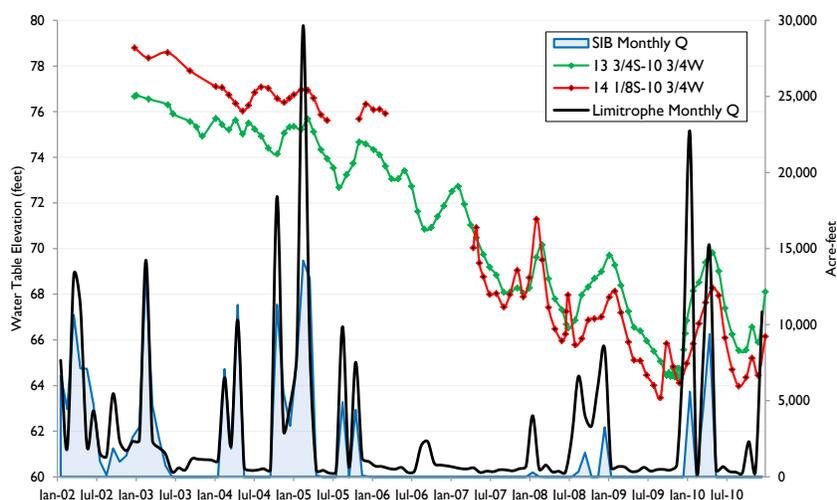
**Figure 53. Water Table Elevation near Hunter’s Hole and Surface Flows, Jan. 2002-Dec. 2010.**
