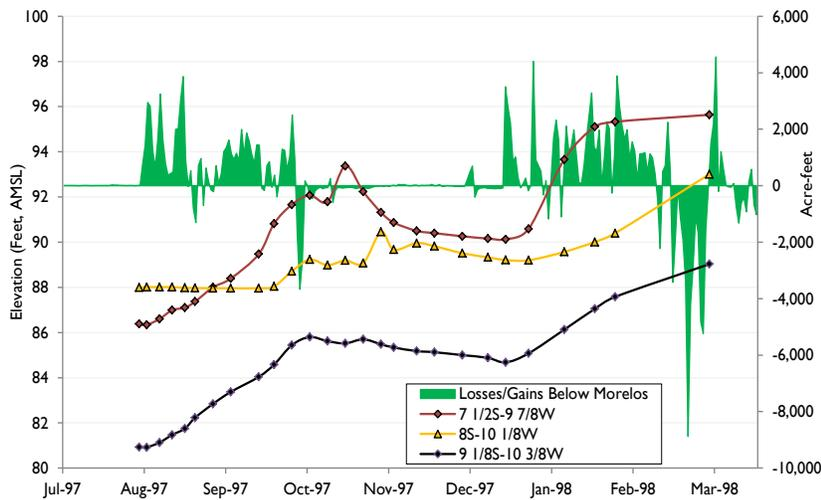
**Figure 55. Water Table Elevations near West Cocopah and Differences between Calculated Colorado River Flows below Morelos Dam and Reported Flows at the SIB, July 1997 – March 1998.**
