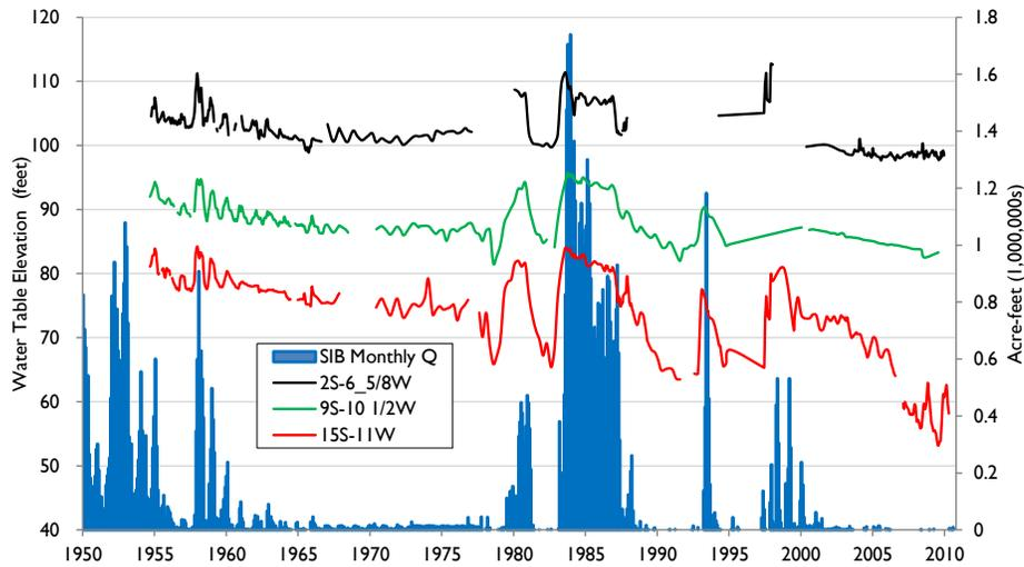
**Figure 49. Water table elevations vs. SIB monthly flows, 1950-2010.** Sources: Reclamation, IBWC.
