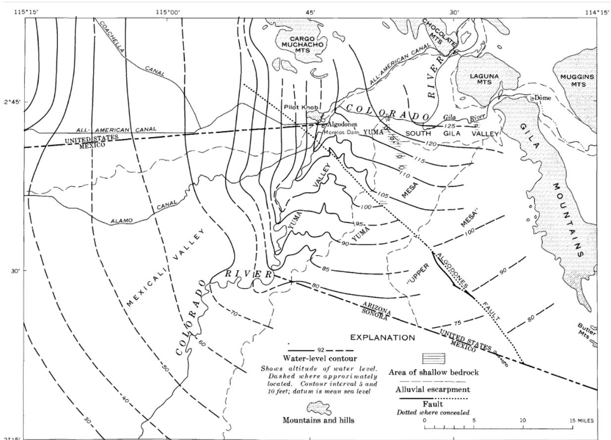
Figure 15. Average Water Level Contours, 1939. Source: Olmsted 1973, Figure 28, p. H86.
