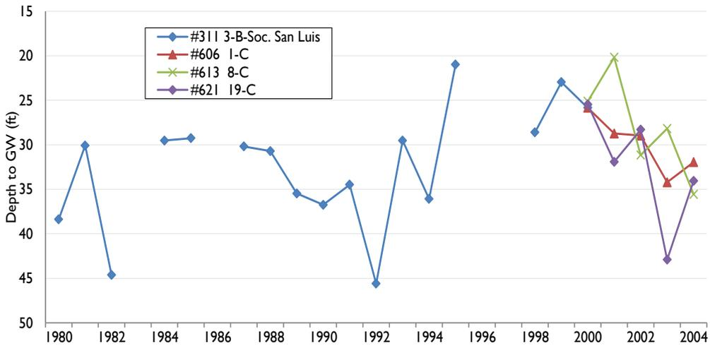
**Figure 23. Depth to Groundwater 1980-2004, west of river channel.**
