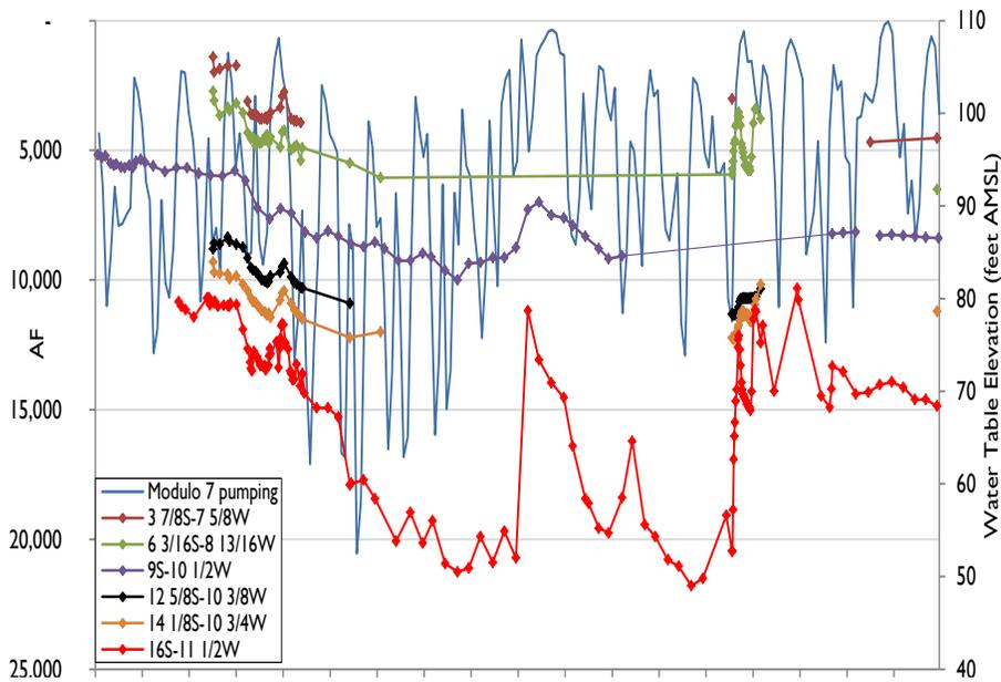
**Figure 38. Reported Monthly Pumping Volumes in Modulo 7 and Water Table Elevations, 1984-2001.** Values on primary y-axis in reverse order. Sources: Conagua, Reclamation.
