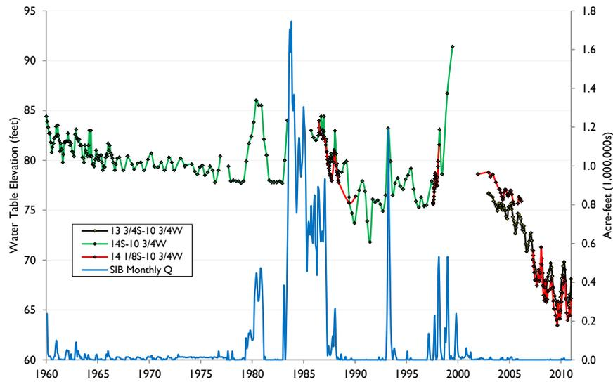
**Figure 51. Water Table Elevation near Hunter's Hole and Monthly Flows at SIB, 1960-2010.**
