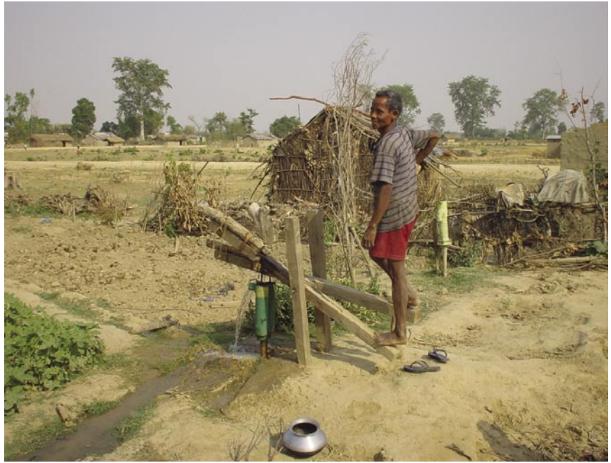
A typical treadle pump. These pumps are cheaper and simpler than motorized devices and have helped millions of farmers around the world boost the amount of water they can give their crops.
