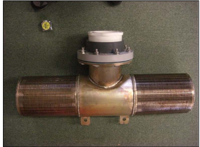
Figure 3. Wedgewire Screen Module Used in Testing During Studies for Santa Cruz and Soquel Creek Water Districts in 2009 and 2010
